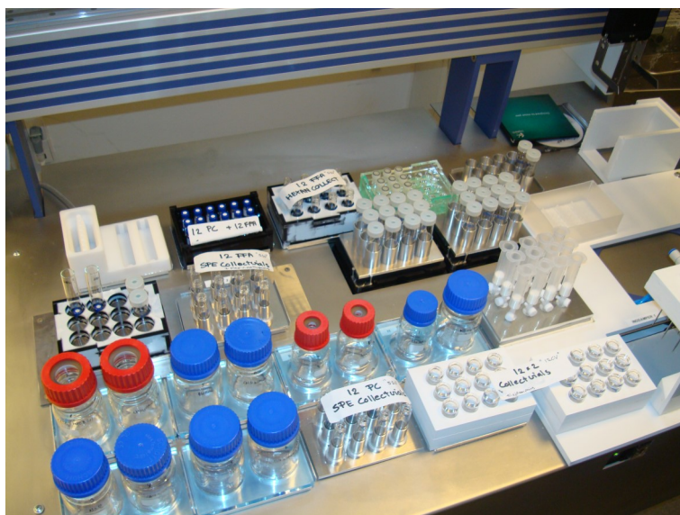
Ex. of setup of different flasks and vials in a compact instrument with under deck centrifuge, SPE and on-line evaporation.
